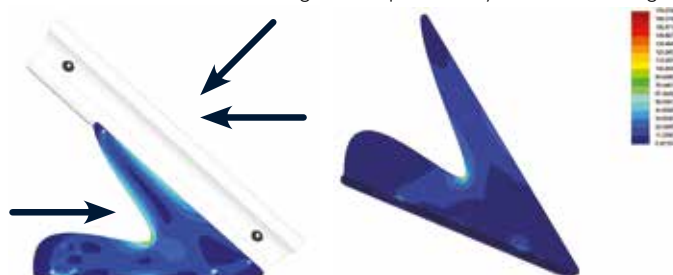
SIMULATION WITH REM ANALYSIS OF WIND AND SNOW LOAD
